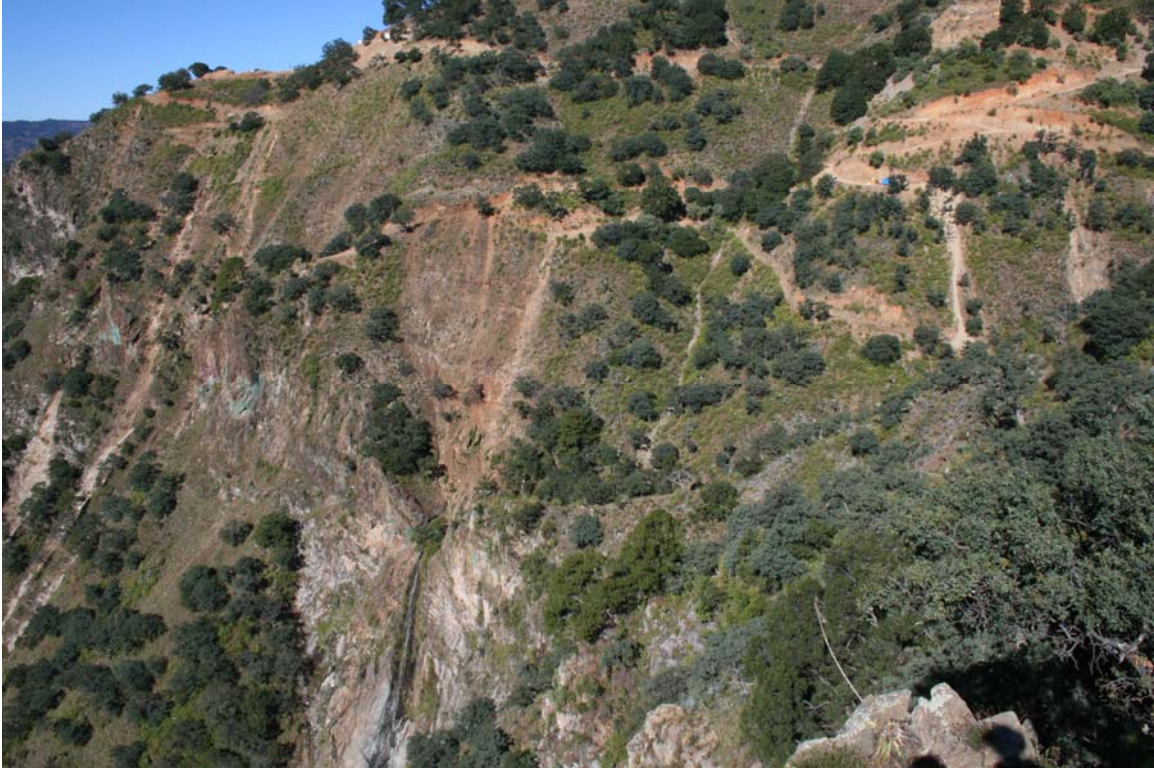
Figure 8. Granodiorite contact with Cretaceous sedimentary rocks occurs at the point of origination of the water falls in lower left central part of the photo. Note green Cuox staining of skarn beds above the contact and presence of drill roads crossing the surface.
