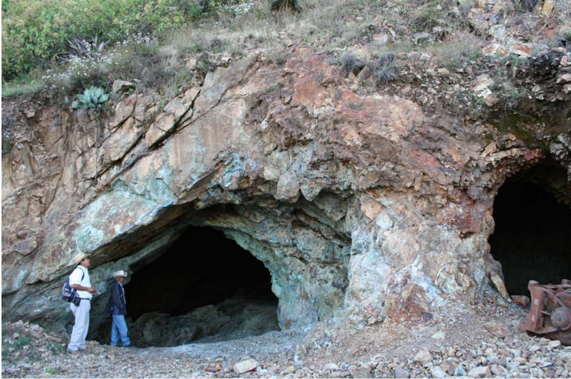
Figure 12. La Incredible mine workings exposing the La Incredible crackle and mosaic breccia with coarse crystalline quartz filling voids. Fault plane over Hector's head is N54E, 29SE. Other structures are E-W, N60E and N20W.
