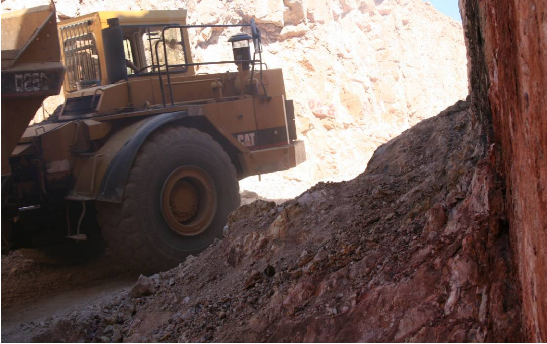
Photo 2. View within the Bamba pit, looking NE along the main San Miguel fault (N40E), which hosts a 3 cm thick quartz veinlet at this point, but silver occurs in the brecciated wall rocks.
